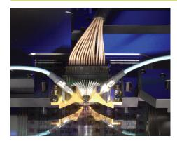
Simultaneous use of DC ProbeWedge and  $\left|Z\right|$  Probes in PA300PS.
